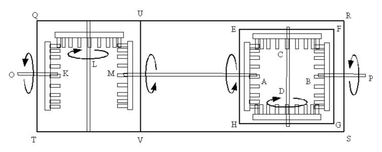
In a chassis QURSVT three gears K, L and M are placed, identical to those of the differential; gear K is fixed to axle OK, gear L turns freely on its axle (one could say that it is a kind of satellite) and gear M is fixed to axle MA. The axles OK, MA and LP are free to turn in the frame members, respectively QT, UV and RS of the chassis.
