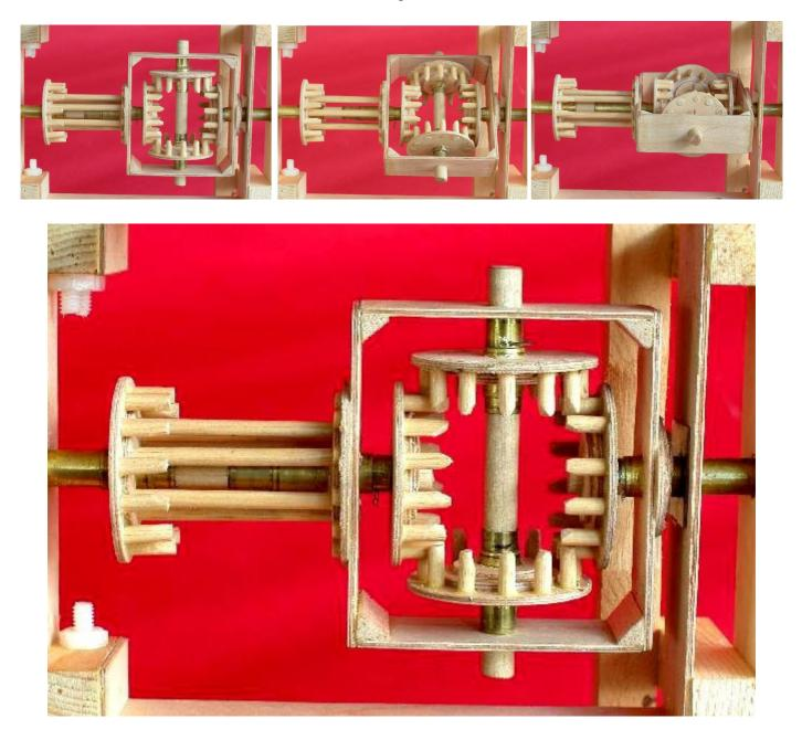
The two gears on the vertical axis must be symmetrical. Concentrate on the four gears on the right of the figure. It has two vertical gears mounted on horizontal axles, these gears are called the "planetary gears"; there are two horizontal gears mounted on a vertical axle but they turn freely on this axle; these gears are called the "satellites".
