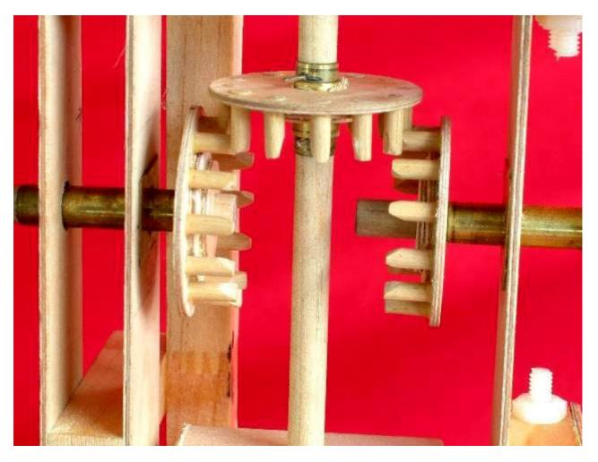
If the left gear turns in a direction, the gear on the right-hand side will turn in the opposite direction.
