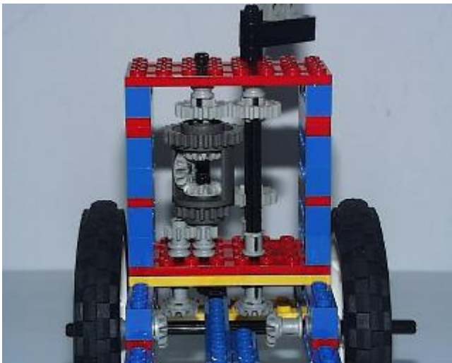
The left wheel connects to the top input axle while the right wheel connects to the bottom input axle of the differential gear.
