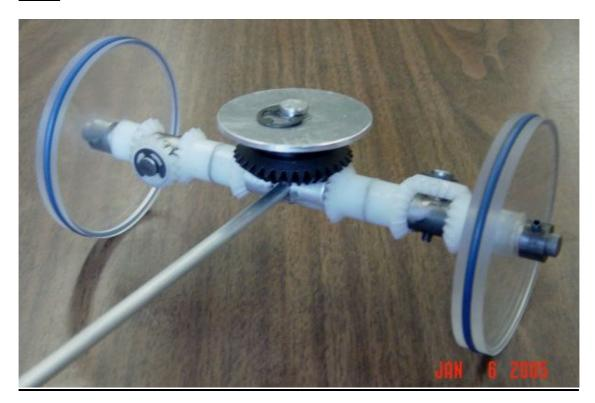
Place the Center Gear and Top Plate in the Center Shaft.
