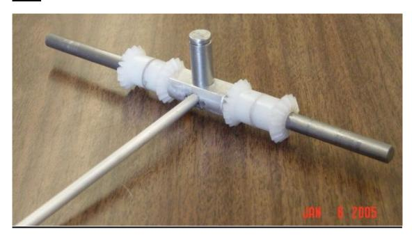
Place the cluster gears on the Main Axle.
