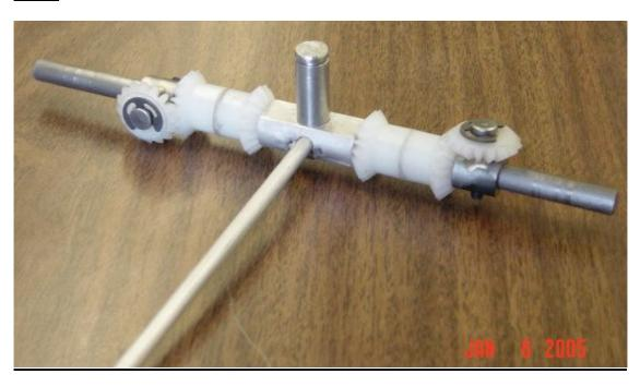
Place the Side Gears on the Main Axle.
