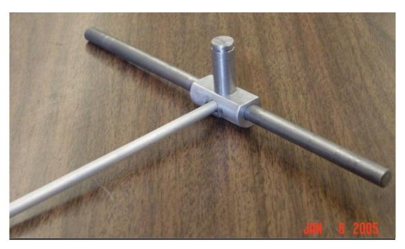
Place the Body, Pull Arm and Center Shaft on the Main Axle.
